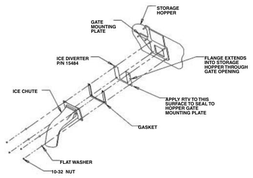
FIGURE 1. Exploded View of Ice Diverter Installation
